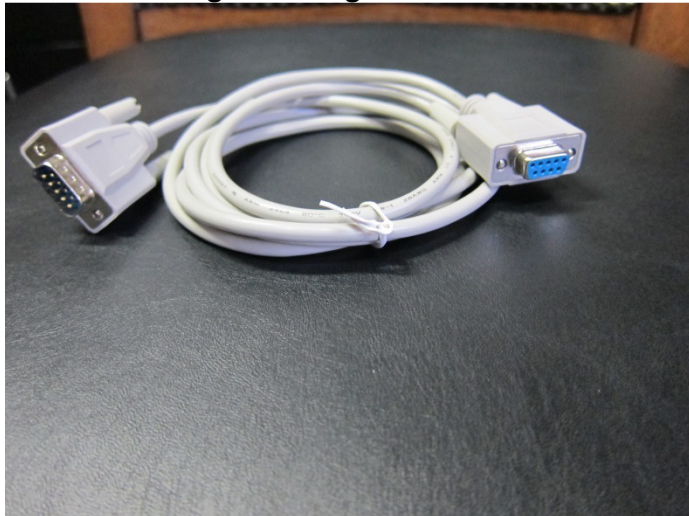
Standard Straight-Through M/F RS-232 Cable
