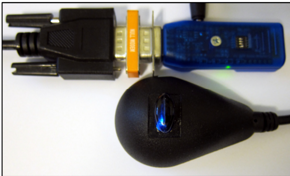
IOGear Bluetooth In USB Dock Serial Cable, 9M/9M NM Adapter, and BlueSnap connected to PCM with External Power
