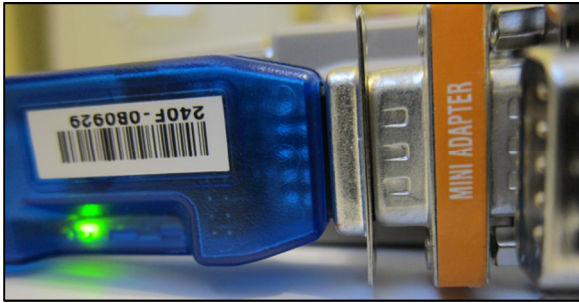
BlueSnap and Mini 9M/9M Null Modem Adapter on Host PCM Port
