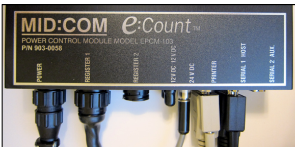
ECount PCM Connections with 9M/9F Straight Cable connected to Mini Null Modem Adapter and BlueSnap connected to PCM w/ PCM External Power
